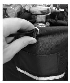
After bag is secure; the oxygen cylinder can be placed inside. Pull the locking cord tight to ensure that tank is secure.
