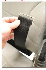
3. Position top Velcro connections at the top of the seatback and hold. Thread metal ring under seatback and bring up the backrest.
