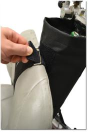
4. Meet metal ring and the bag at the top of the seatback. Feed top Velcro attachment through the metal ring.
