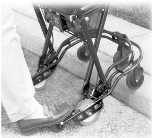
After raising the front end, release the brake and roll up the obstacle. This feature requires reasonable balance and is not appropriate for everyone. If you feel unsafe using this feature, keep the locking pins in place.
