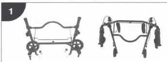
Remove rollator frame 1 from box and lay on flat surface.
